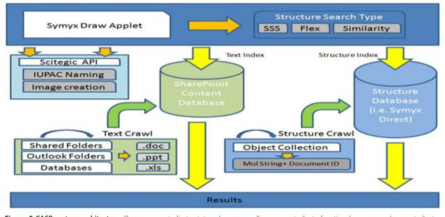
Figure 5 CASP system architecture. Orange arrow indicates internal process; yellow arrows indicate functional process, and green indicates nightly process.
