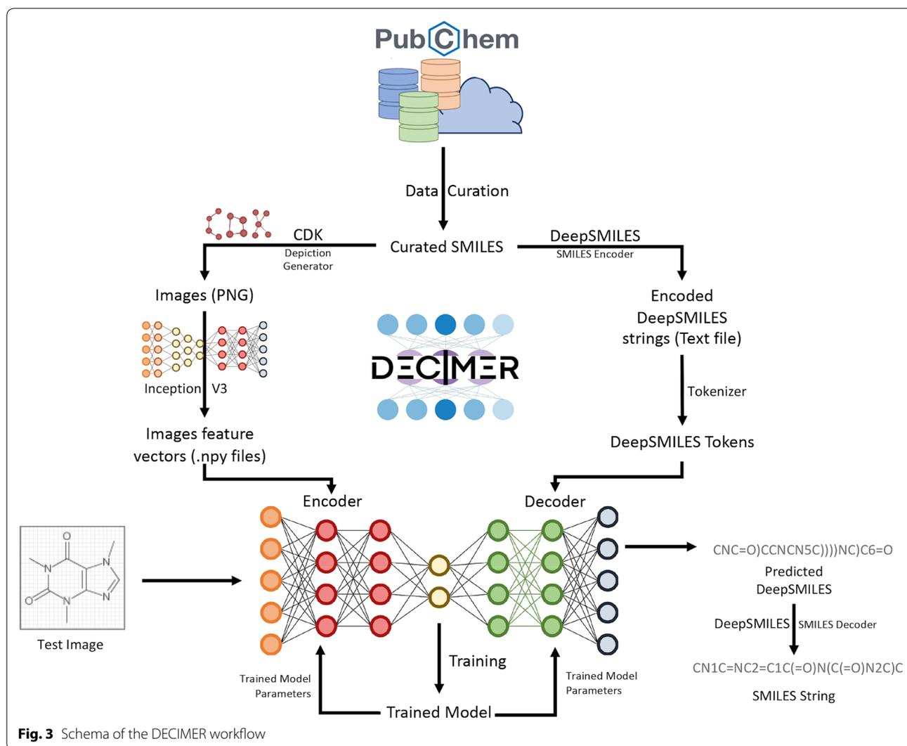
implementation of Show, Attend and Tell, published at [23], which is used unaltered by us. Their encoder network is a convolutional NN (CNN), which consists of a single fully connected layer and a RELU activation function. Their decoder network is a recurrent NN (RNN), consisting of a gated recurrent unit (GRU) and two fully connected layers. The soft attention mechanism used in [23] was introduced by Bahdanau et al. [24].
