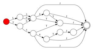
Fig. 15 DFA that matches WLN strings for Benzene, Cyclopenta-1,3-diene, Cyclohexane, Cyclopentane,4 H-indene and Hexahydroindan. Root state is given in red, with the only accept shown with a double circle
