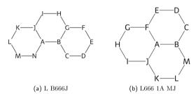
**Fig. 7** Locant Paths shown on chemical structures for **a** Phenanthrene and **b** Phenalene. WLN alphabetic indexing is shown on each atom. For Phenalene, the highest priority atom is the perifused center, and therefore it takes the starting point. Any further peri-fused points will force the path to travel in that direction
