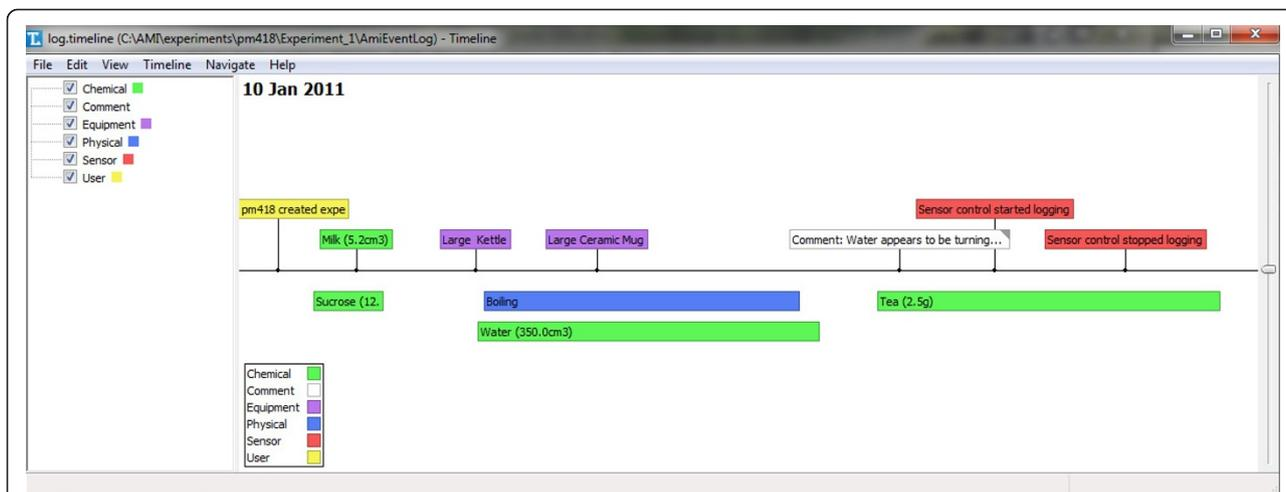
**Figure 7** Graphical view of experiment timeline. The Timeline application [31] is written in Python and receives an XML event-log file created by Ami. Timeline takes this event log and displays different sorts of events in different colours.
