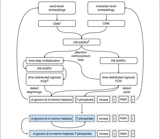
**Fig. 2** Model architecture. The figure illustrates the topology and of the best-performing full-featured model. <sup>1</sup>CNN convolutional neural network; <sup>2</sup>HS-biGRU half-stateful bidirectional gated recurrent unit; <sup>3</sup>FCN fully-connected network
