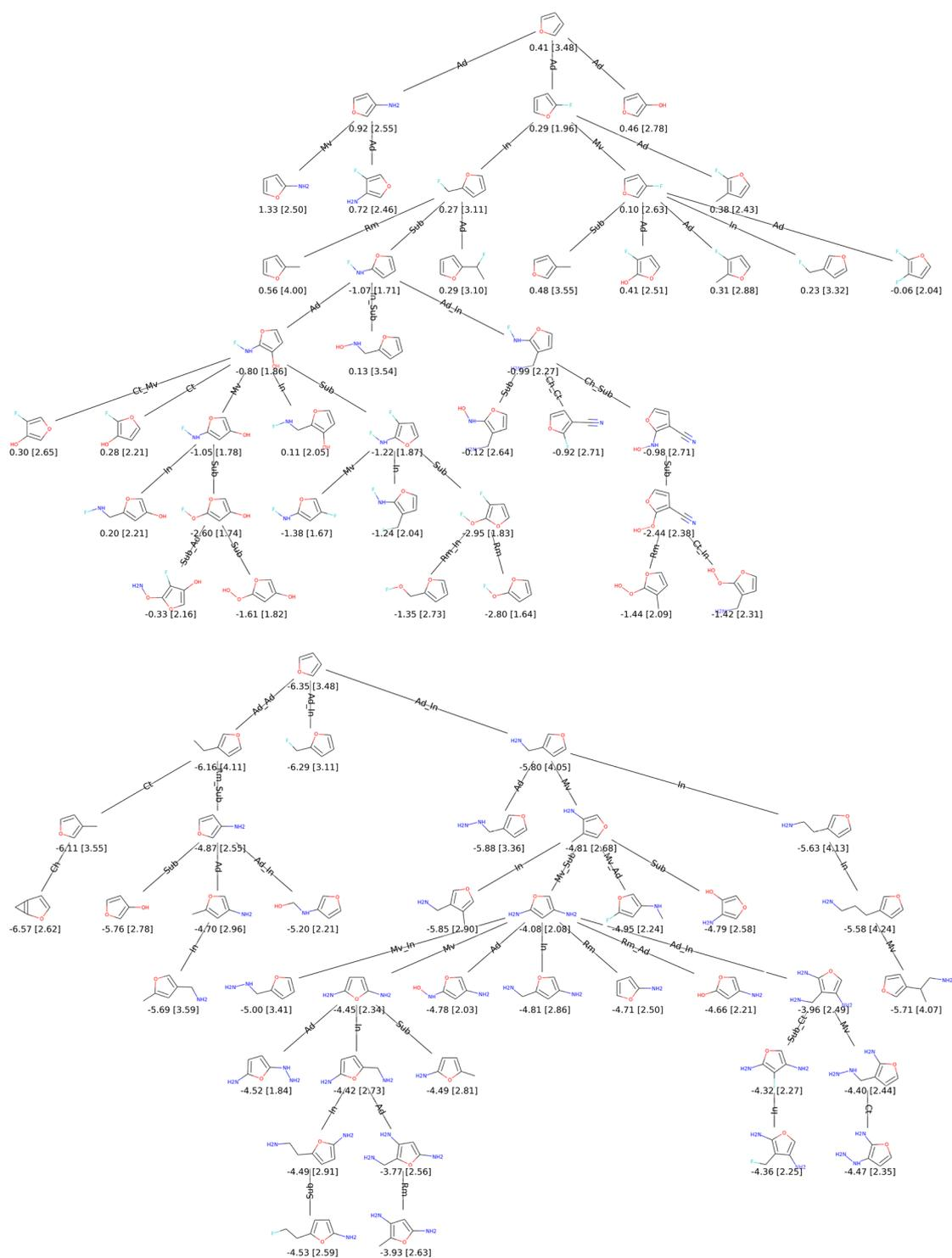
**Fig. 10** Exploration trees for the minimisation of LUMO (top), and the maximisation of HOMO (bottom) energies starting from a fixed furane core. Energy values (in eV) and [CLscores] are reported under the solutions. The actions used for the transition between two molecules are reported on the edges with the following legend. Ad: append atom, Rm: remove atom, Ch: change bond, Sub: substitute atom type, In: insert carbon and Mv: move group
